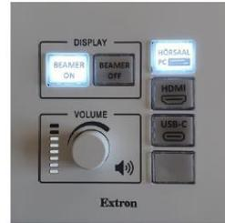
**Projector:** Press **BEAMER ON** to power up the projector and **BEAMER OFF** to shut it down.
